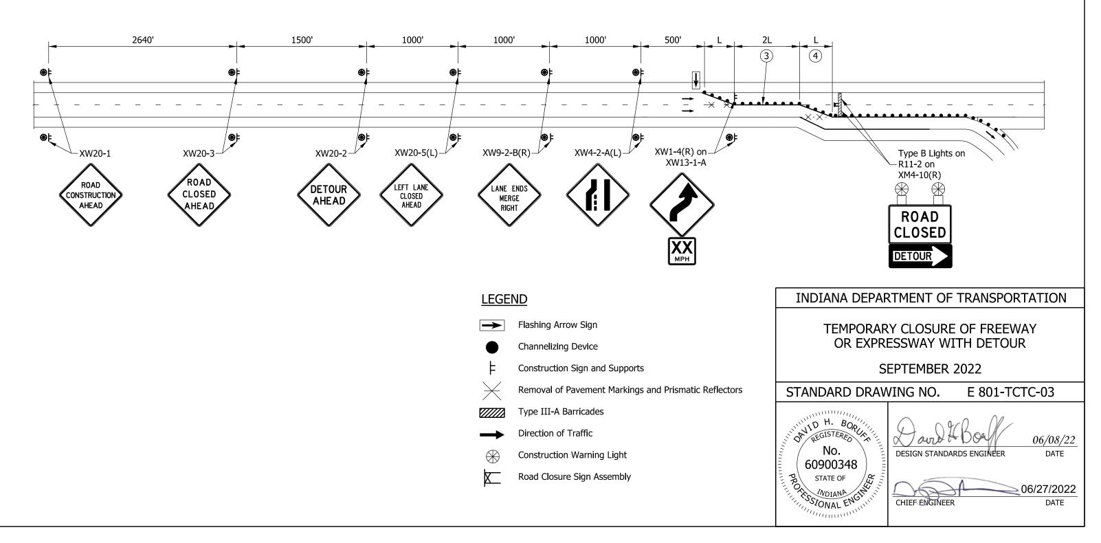
1. See Standard Drawing E 801-TCDV-03 for merge distance, L. The value of L on freeways shall be based on 70 mph.
